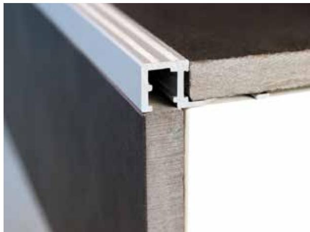
SQUAREJOLLY SJR with Resin Grip is a square section profile designed to finish and protect the tile's edges from shock and mechanical impact. Minimalist and modern design, ideal for residential projects. The resin stripes on the upper surface make the Squarejolly SJR anti slip, certified R11. The profile is also resistant to abrasion (PEI 3) and to chemical agents.
